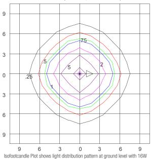
Isofootcandle Plot shows light distribution pattern at ground level with 16W LED light engine. Readings have been taken assuming the photometric center of the luminaire to be 3.29 feet above ground level. IES files for standard lamps are available on our website.
