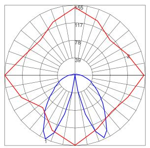
Maximum Candela = 155.4; Located at Horizontal Angle = 180; Vertical Angle = 25 #1 - Vertical Plane Through Horizontal Angles (180 - 0) (Through Max. Cd.) #2 - Horizontal Cone Through Vertical Angle (25) (Through Max Cd.)
