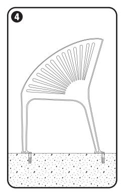
• Position bench so that mounting holes line up with anchors.
