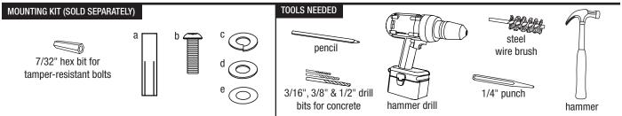
STEP BY STEP FOR ALL SURFACE MOUNTED CORDIA BENCHES (SBCOR-72B SHOWN)
