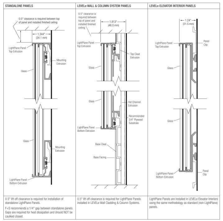
If LightPlane panels are installed in third-party frames, a minimum clearance of .125" is required on each side of the panel for assembly tolerance and thermal expansion of materials.
