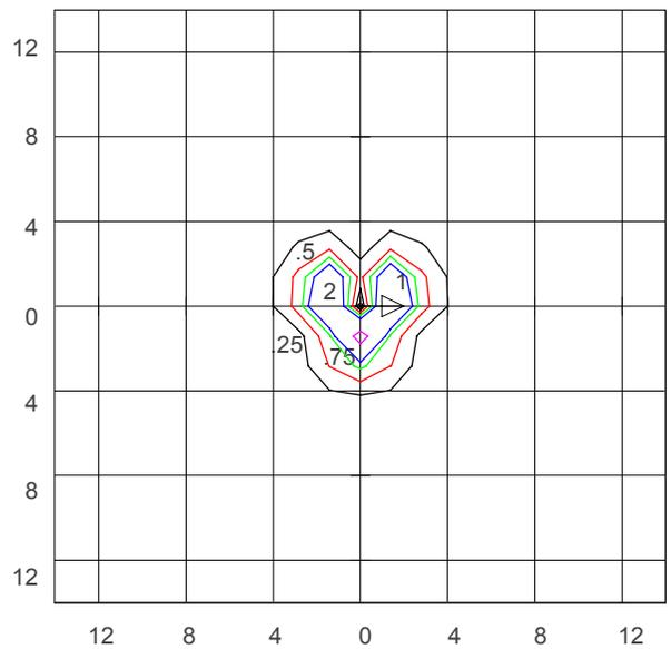
Isofootcandle Plot shows light distribution pattern at ground level with custom LED light engine with no shield. Readings have been taken assuming the photometric center of the luminaire to be 2.74 feet above ground level. IES files for standard lamps are available on our website.
