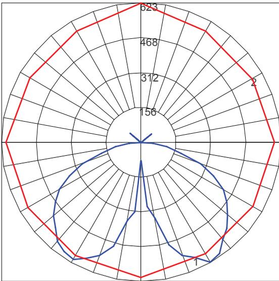
Maximum Candela = 623.46; Located at Horizontal Angle = 90; Vertical Angle = 30
