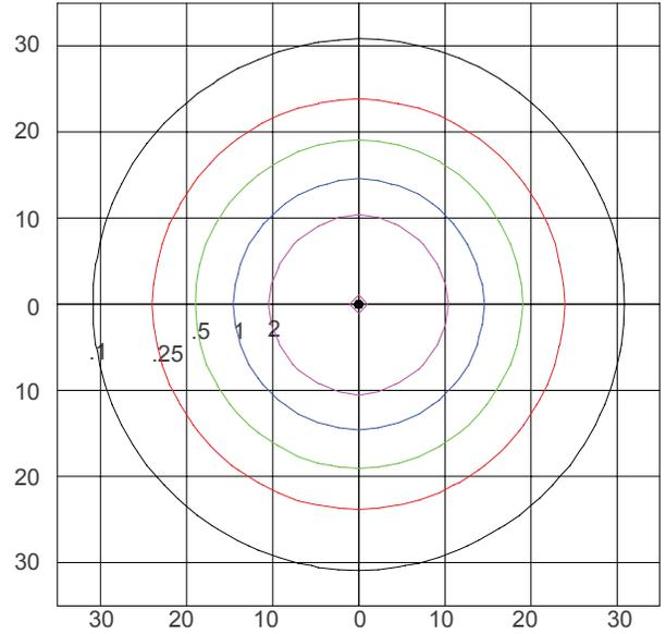
Isofootcandle Plot shows light distribution pattern at ground level with LED chip with no shield. Readings have been taken assuming the photometric center of the luminaire to be 11.13 feet above ground level. IES files for standard lamps are available on our website.
