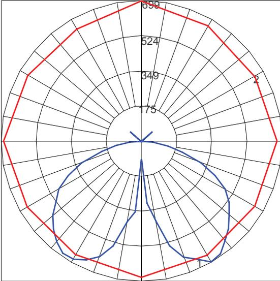
Maximum Candela = 698.91; Located at Horizontal Angle = 90; Vertical Angle = 30
