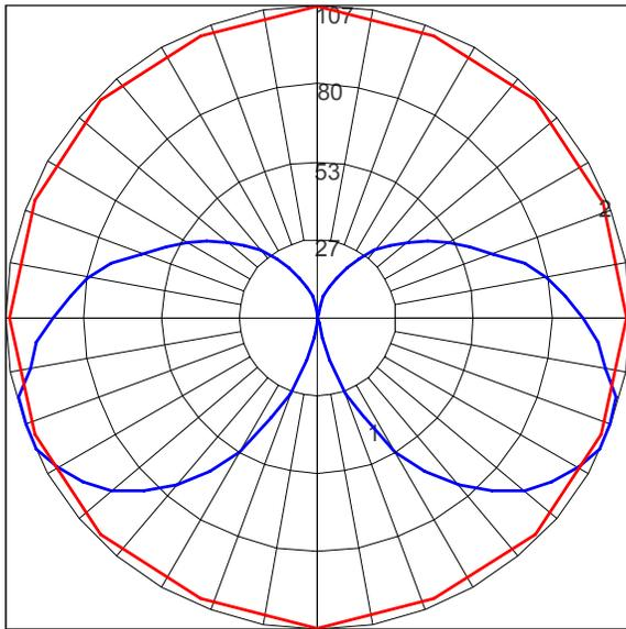
Maximum Candela = 106.94 Located at Horizontal Angle = 90, Vertical Angle = 70
