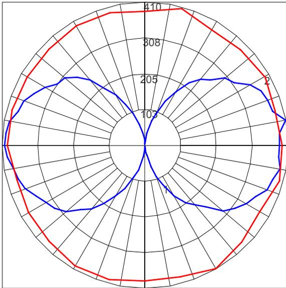
Maximum Candela = 410.2; Located at Horizontal Angle = 300; Vertical Angle = 100
